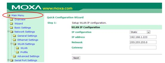
The Wizard of our Moxa device included settings for Operation Mode and TCP Port – but, in our case, we still had to confirm/adjust the Application, Mode and TCP Port via the serial port settings shown below.
