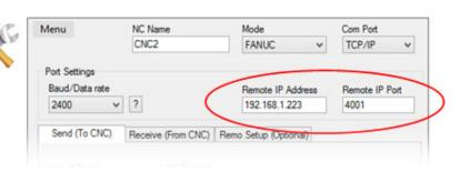
Note: When transmitting over IP the DNC speed is no longer relevant. However, setting the DNC speed to the same speed as the Serial Device Server will improve the visual display of the DNC software. It can also reduce volume network traffic and prevent buffer-full events in the serial device server.
